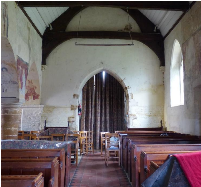
Tower curtains and external door curtains can significantly reduce air movement and draughts.
