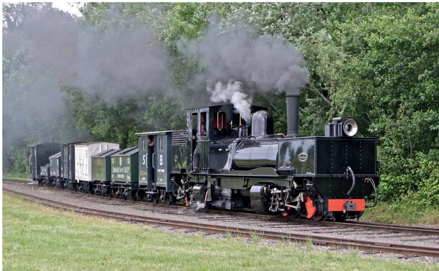
*Based on the Statfold Barn Railway is the Tasmanian Government Railway K1, built by Beyer, Peacock in 1909. It's depicted working a narrow-gauge goods train between the Loop and Statfold Junction on 11/6/22.*
