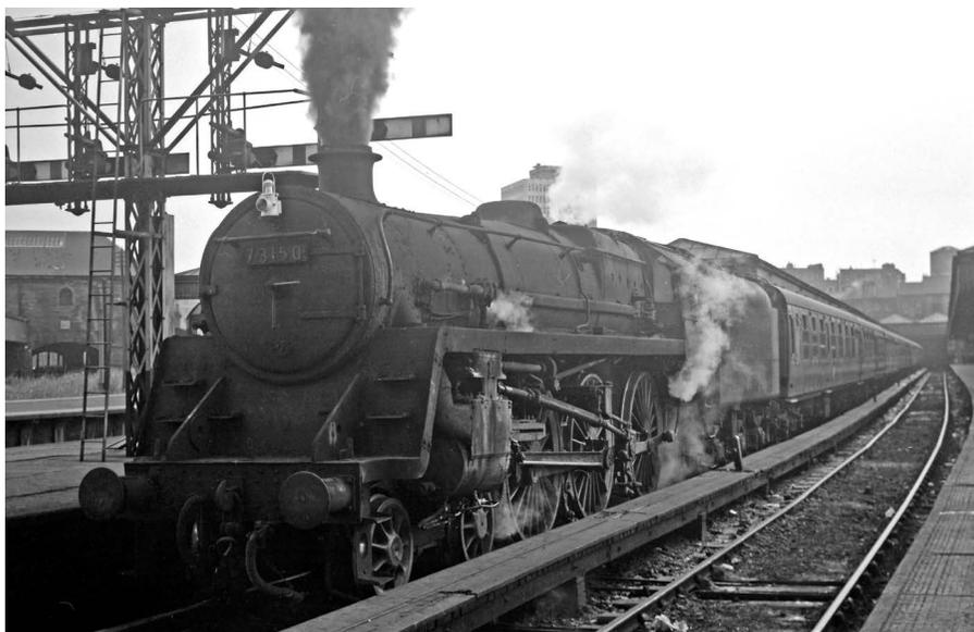
*Next to the A4 is BR Standard 5 4-6-0 73150 with Caprotti valve gear, taken on the same day as the A4, in early September 1966. The destination of this service was not recorded.*
