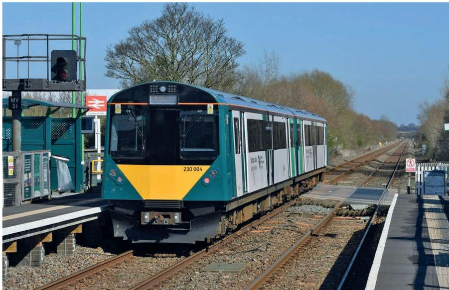
*Services on the Bletchley to Bedford line, suspended during Covid, are operating once again albeit to a reduced frequency. The attached picture shows 230.004 departing from Kempston Hardwick Halt for Bedford on 19/3/22. There are three of these DEMUs, converted from ex-LT D78 stock, at Bletchley.*
