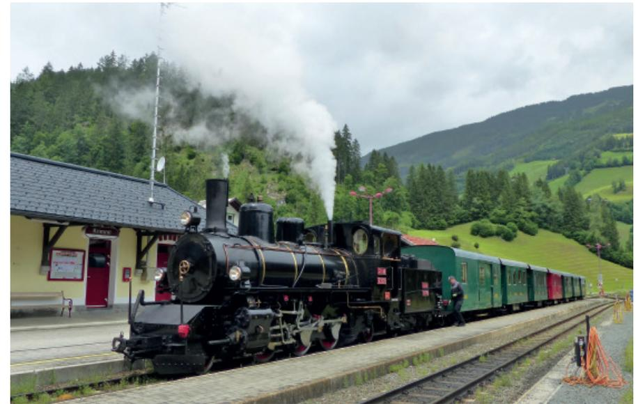
*Austria. Member Elnar Pfannerstill took this photo on 15/7/21 just before the awful floods destroyed a large part of the rail and this station was later encircled by a landslide. Former JZ 760mm gauge 2-6-2 73-019 (Bp 3287/1913) has just arrived at Krimml with the tourist train from Zell am See.*
