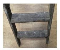
This ladder was condemned for the state of its treads and a split in one of its stiles.
