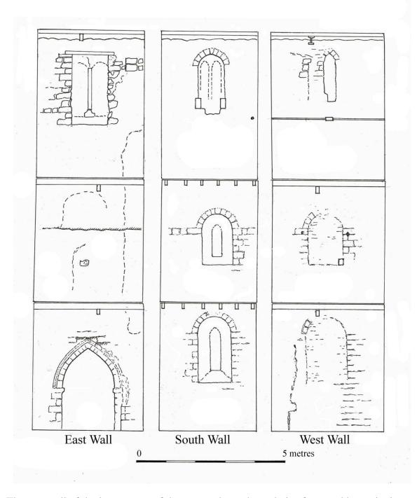
The east wall of the lower stage of the tower, above the arch, is of coursed but quite irregular fabric, in contrast to the other three walls which are of better-coursed diagonally-tooled stone
