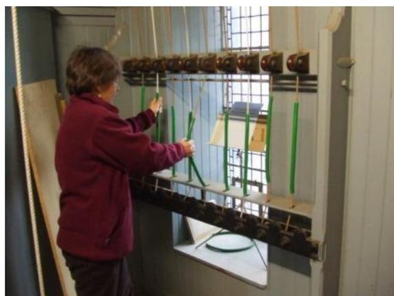
Fig. 6. An Ellacombe hammer and rack (here for 10 bells)
