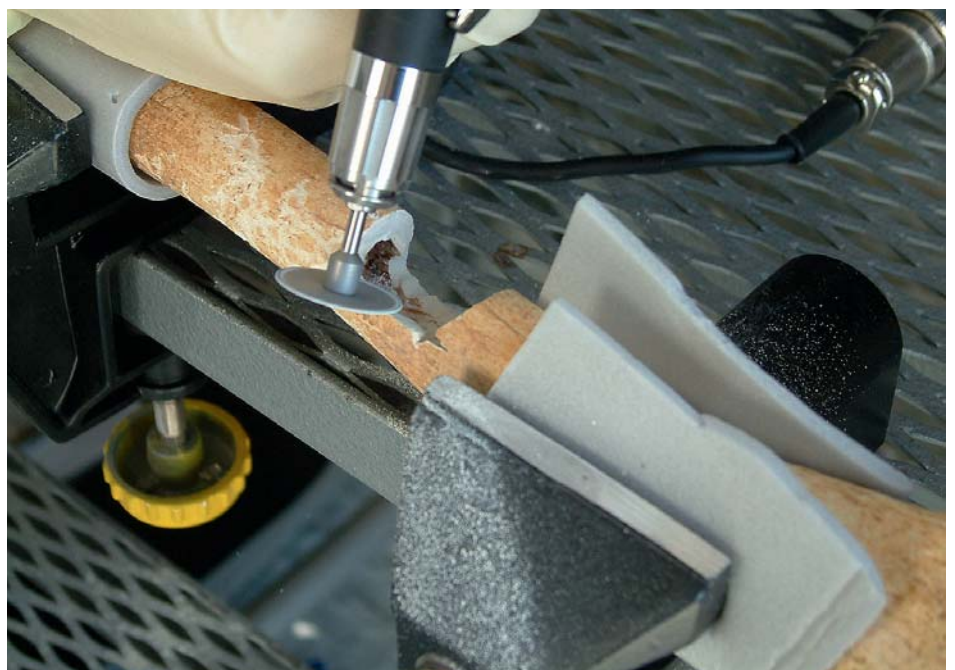
Fig 1 A sample being cut from a femur for radiocarbon dating. The bone is held in two small vices, padding being used to prevent damage to the specimen. The small rotary electric saw has been used to remove the sample.
