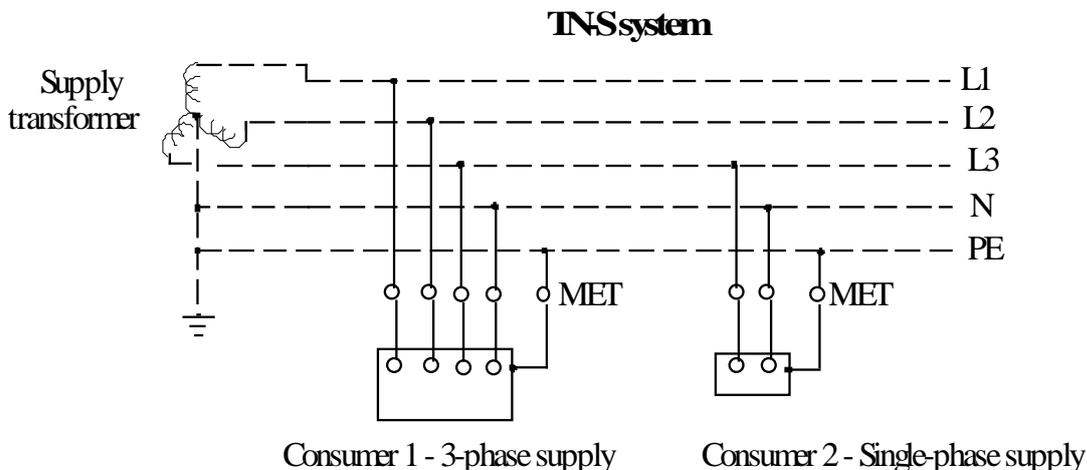
In a TN-S system there are separate neutral and protective earth conductors throughout, i. e. in both the supplier's distribution in which the metallic sheath of the cable is earthed and in the consumer's installation. The consumer is therefore able to use the supply PE conductor via a connection to the MET.
