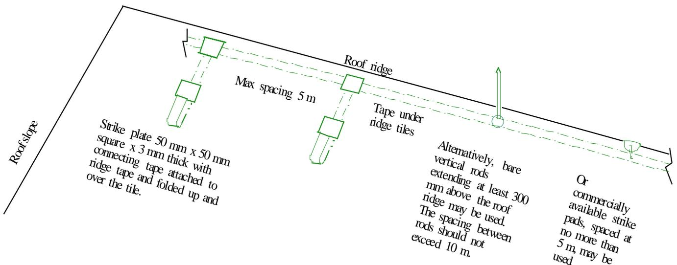
**Figure 2 – Air terminations for ridge conductor placed under the ridge tiles**
