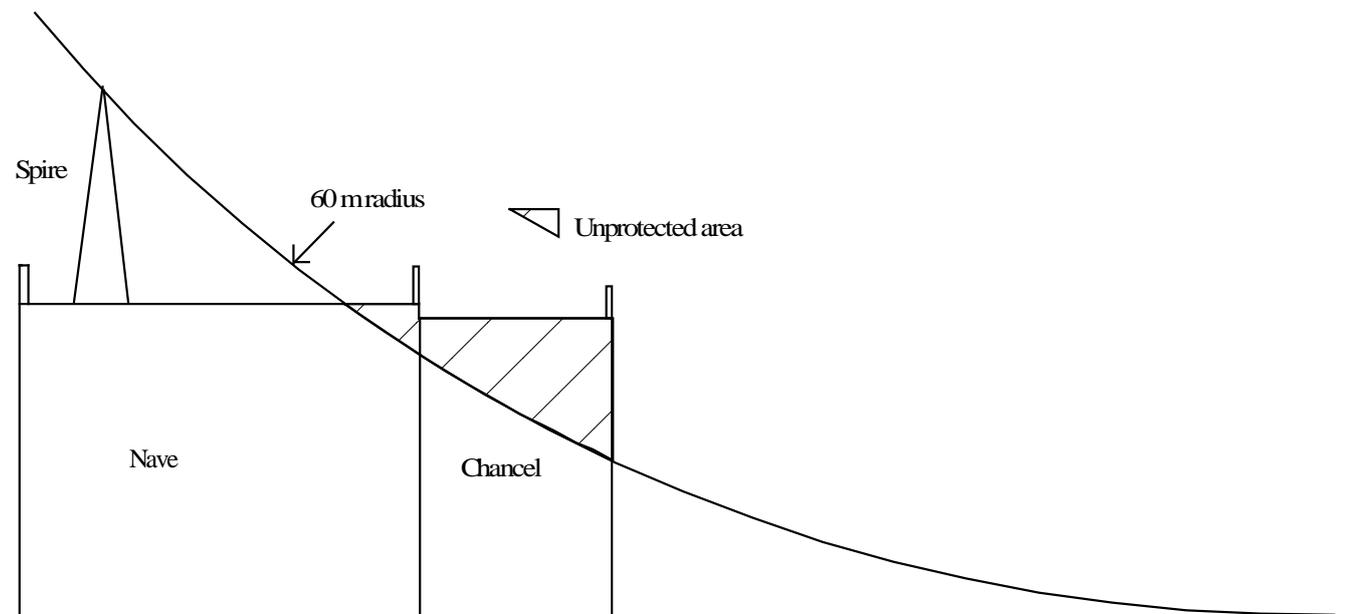
**Figure 1 – Unprotected area with spire-only protection**
