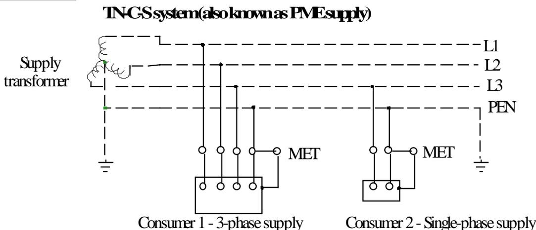
In a TN-C-S system the neutral and protective functions are combined (C) in a single protective earth and neutral (PEN) conductor in supplier's distribution. The system is also known as a protective multiply earthed (PME) system, as additional earthing, say at every third pole of an overhead supply, guards against a hazard arising from the unlikely event of a broken neutral.
