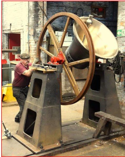
*Above: An image showing a bell being analysed in our testing stand.*
