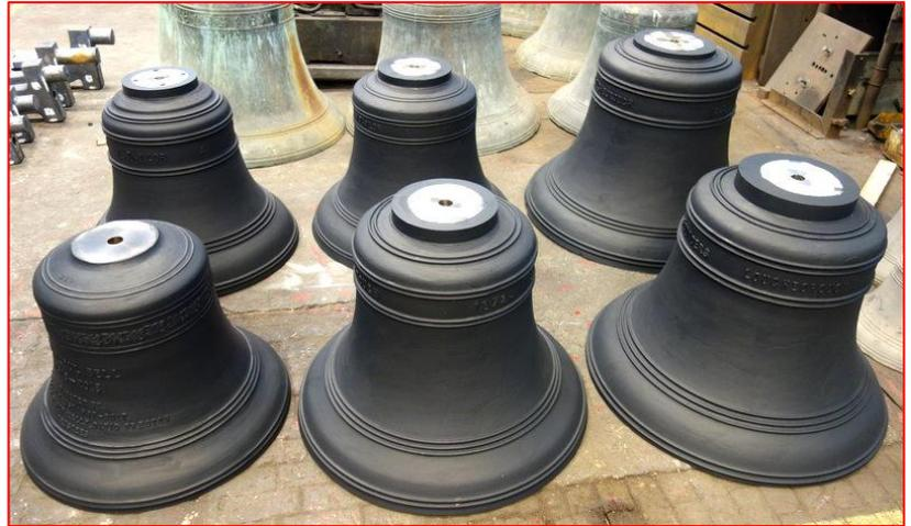
*Above: An image showing a peal of bells which have been tuned, had their canons removed, had resin pads cast upon their crowns and have received their first coat of polish. Ready to receive their new bell fittings.*
