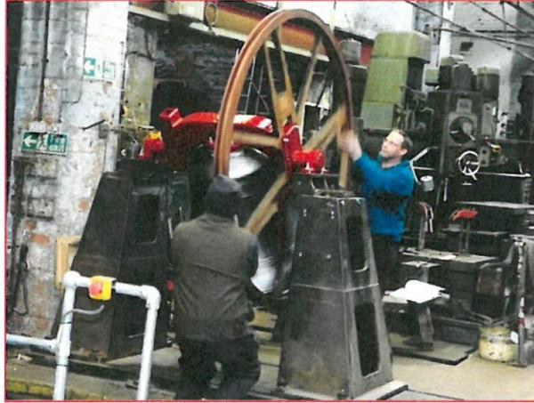
*Above: An image showing a refurbished bell being swung in our testing stand.*
