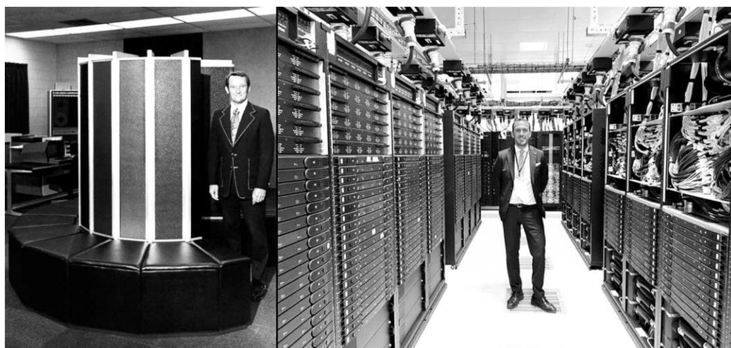
The Centre started with the most powerful computer available in 1975, a 'Cray 1' (shown on the left with the designer). Today a mobile phone would have several times the processing power!
