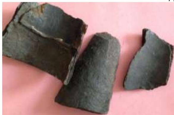
*their inner surface, ruining the integrity of the pipes. It was also discovered that, under normal conditions, they were susceptible to collapse under applied loading sooner than pipes made of more rigid materials.*
