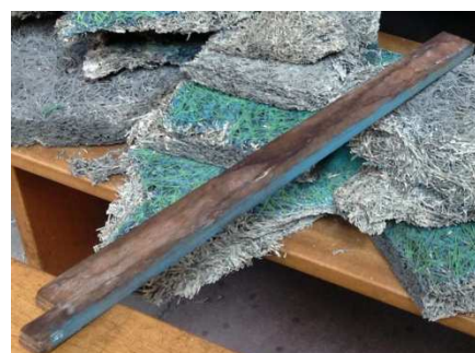
Figure 4. Fragments of wood wool and plywood battens recovered from the collapsed section of the ceiling
