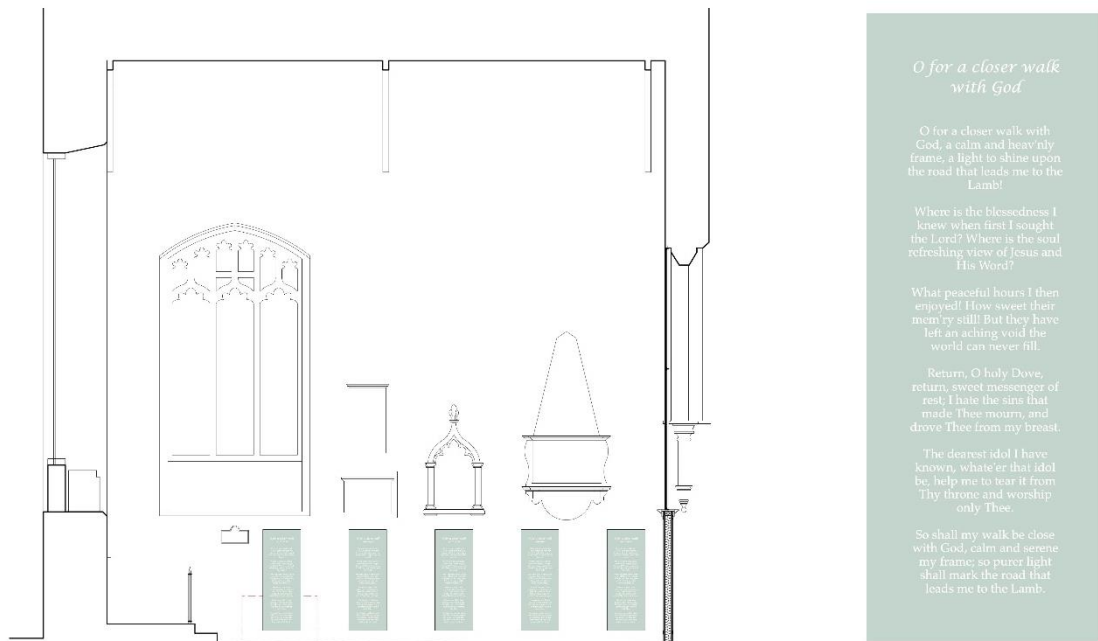
Figure 36 The East wall of the Cowper Room showing the proposed arrangement of radiant panel heaters that will also function as interpretation panels of the life and writings of William Cowper.
