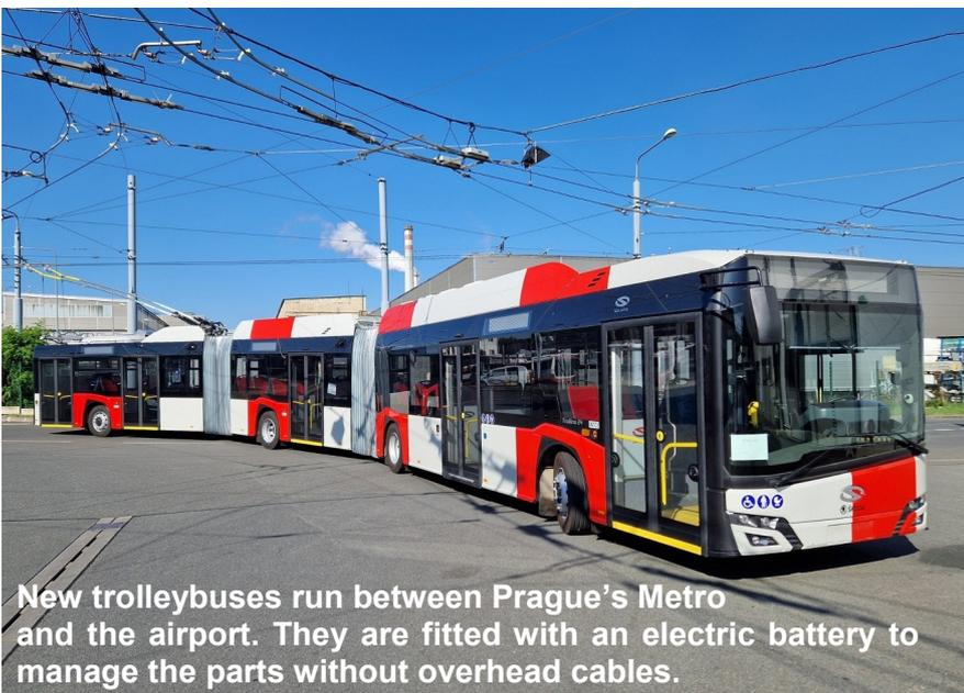
New trolleybuses run between Prague's Metro and the airport. They are fitted with an electric battery to manage the parts without overhead cables.
